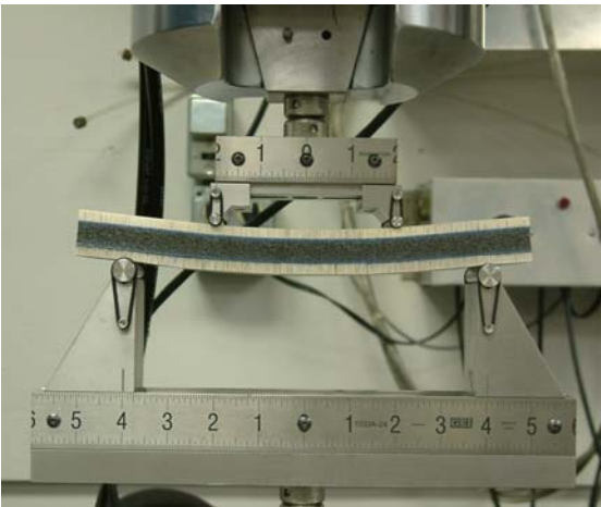
Figure 4 – Carbon Foam/E-Glass/Balsa Core
