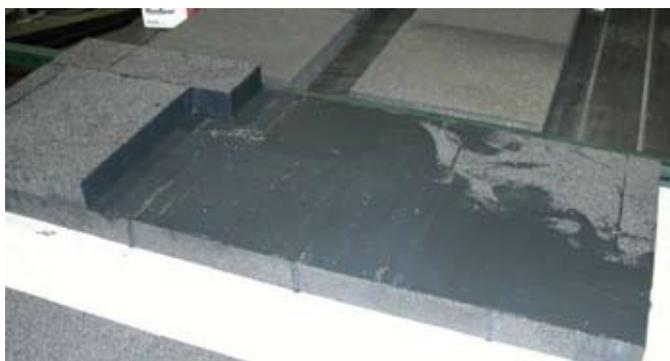
Figure 8. Coal-based carbon foam bonding adhesive.
