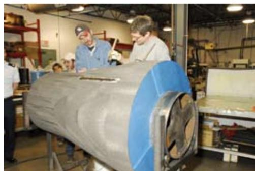
**Figure 19.** Installation of thermocouples and chopped carbon surface.
