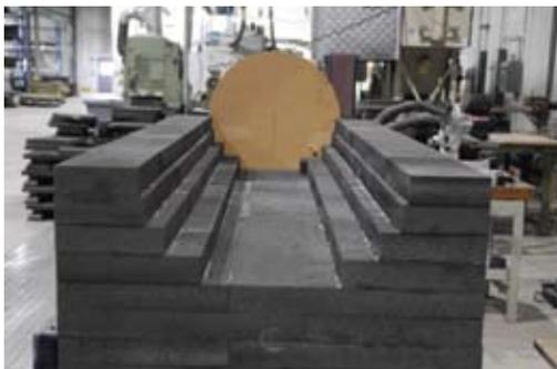
**Figure 16.** Coal-based carbon foam blocking and rough lay-up.
