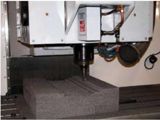
**Figure 10.** Coal-based carbon foam rough machining.
