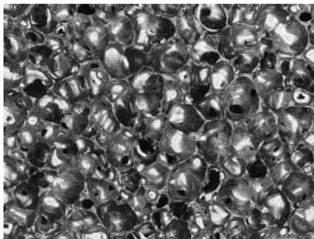
Figure 2. Coal-based carbon foam microstructure.
