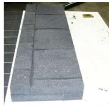
Figure 9. Bonded coal-based carbon foam billets.
