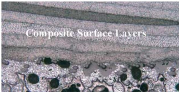
Figure 4. Coal-based carbon foam SEM image.
