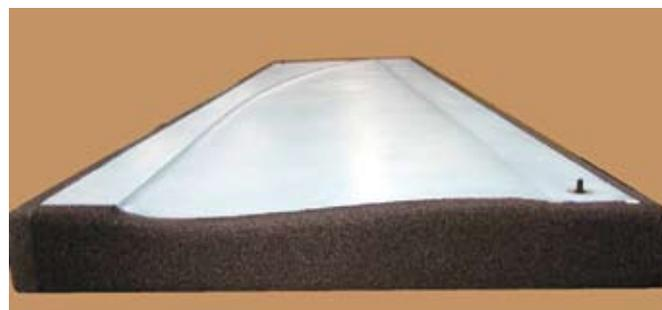
Figure 6. Coal-based carbon foam-prototype tooling.
