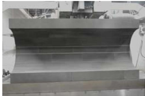
**Figure 17.** Coal-based carbon foam inside mandrel rough machining.
