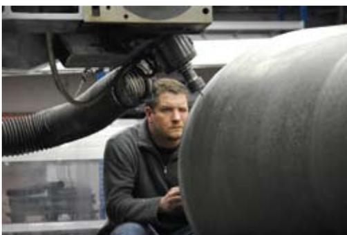
**Figure 20.** Machining of chopped carbon surface.
